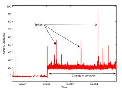
Figure 4: One month of CPU utilization in a backbone router
